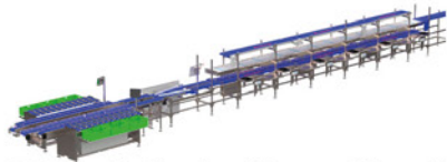
IPS: Line with 4 levels and front weighing tables and MHP 3000 semi-automatic combination scale
