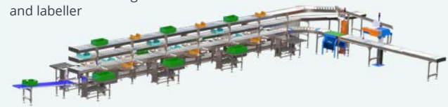
IPS Frontal weighing tables with 4 levels of conveyor lines, automatic checkweigher and labeller
